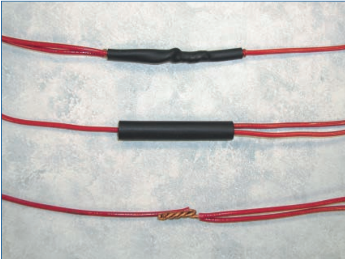
Meltable inner liner for encapsulating
